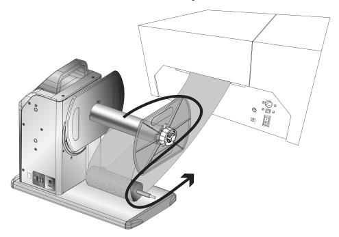
3. Open the Cover. Install an empty core in the LX2000 which is equal to or greater than the width of your label stock. Feed the stock into the printer between the Fixed Throat Guide and the Movable Throat Guide.
