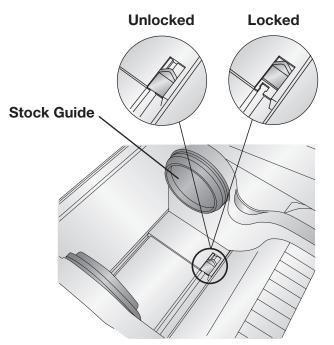
2. Load the label stock as shown. Feed the stock through the opening in the back of the printer. The UW-7 should be as close to the printer as possible without causing interference with the dancer arm. Manually move the dancer arm up and down to ensure that it will not touch the printer.
